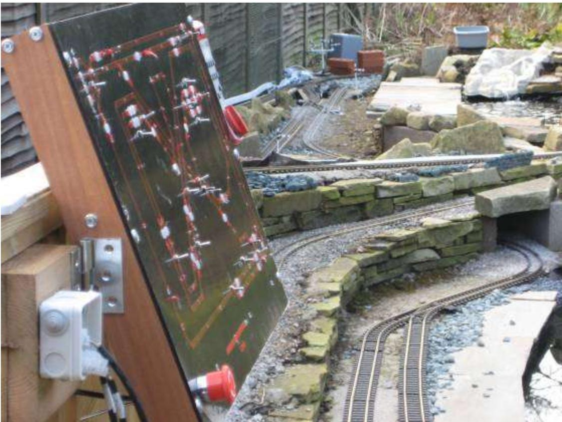
View of the layout from the decking. Control panel in foreground and signals beyond. The big RED button is the signalman's emergency stop button and cuts all power to the track.
