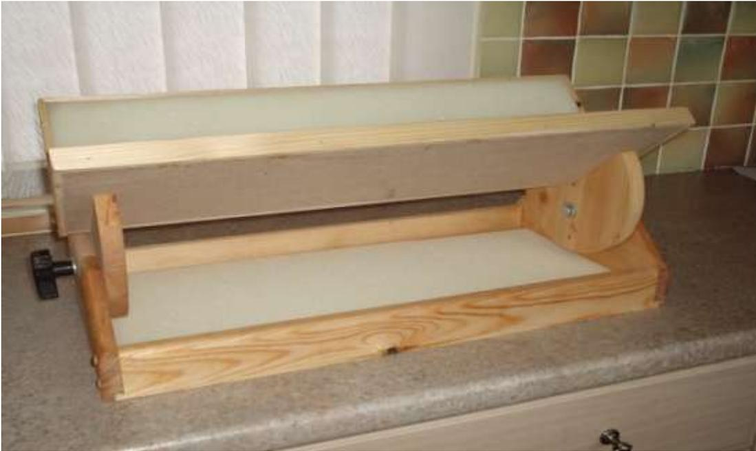
Fully assembled work station with knurled knobs for adjusting for angles.
